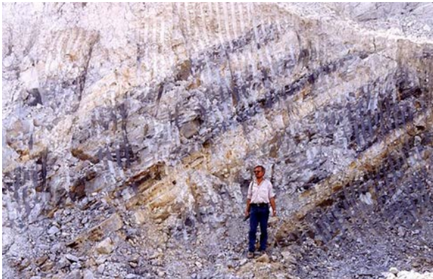
Figure 3. Saprolite of the Mesozoic–Tertiary weathering mantle with interfingered transition between the white, bleached oxidation horizon and the black reduction horizon below. The saprolite of both horizons displays a well-preserved rock structure, but it is soft and friable.
